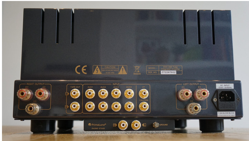
Gold-plated heavy-duty WBT style multiway speaker sockets use solid shafts for better conductance, with 4 and 8 ohm taps on offer. RCA inputs are of equal equality and well spaced
