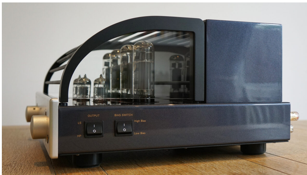
Right side panel hosts switches for headphone or loudspeaker outputs and high or low biasing, making valve rolling a cinch
