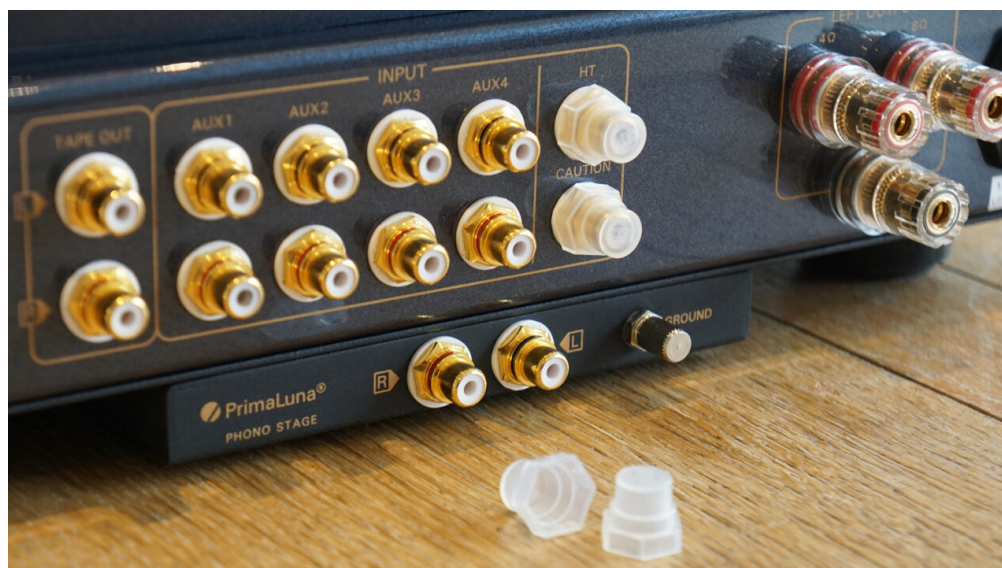
Optional moving-magnet phono stage sits in a separate shielded case that's bolted to the amp's underside. Dust caps are a great inclusion to keep the input sockets clean and protected when not in use
